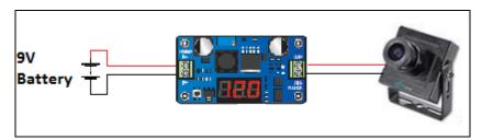
Probably the simplest use for the booster is to increase your power supply voltage if you do not have the correct voltage power supply or perhaps you want to use a battery for testing. Just make sure your power source can supply enough current.
