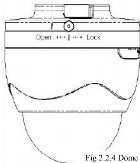
Fig 2.2.4 Dome camera fixed
