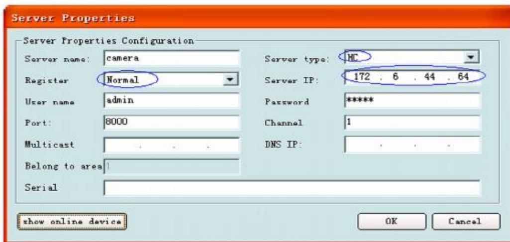
Fig. 5.1.1 Static IP Configuration dialogue box
