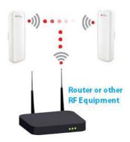
5. It is common that other RF equipment can interfere with the IPmitters, as the IPmitters use the same frequencies that routers and other WiFi equipment uses. This will reduce the range of the IPmitters and reduce the performance. Check the WiFi channels being used nearby to the IPmitter, or avoid placement of the IPmitters near other RF equipment and routers.
