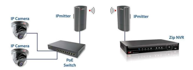
When pairing, one unit needs to be set to "Client" and the other unit needs to be set to "Host".
