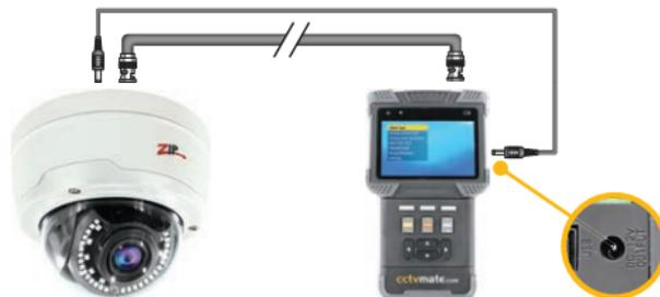
**Note:** *The maximum 12V output is 2A. If this is exceeded the output will be terminated automatically.*
