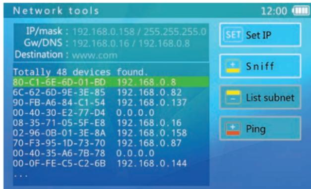
**Note:** *It may take up to 60 seconds for a device to be discovered. As the test listens for any data packets it may find devices with different subnets. The test can not discover silent devices or uni-cast (point-to-point) packets.*
