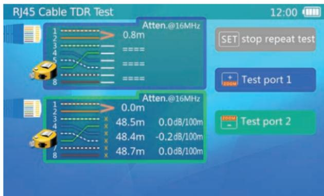
Pressing the 'SET' button will start and stop the 'Repeat Test'. While the repeat test is running the LCD400K will repeatedly test both network ports. This is a great way to test multiple cables quickly.
