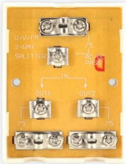
A highly recommended piece of kit when installing a modulator. The DC combiner merges the modulator's output with signal for the TV aerial. This is the most efficient way of integrating a modulator into a household TV system.
