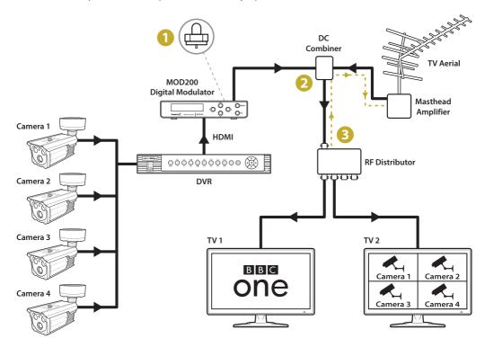
**1** Fit the supplied 75 $\Omega$  RF terminator to the unused RF input on the first MOD200.
