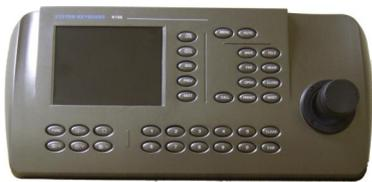
The dome is controlled by an RS485 data signal that is produced by the PTZ715 keypad or a compatible DVR. This data signal tells the dome to pan, tilt, zoom etc.
