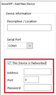
TIP: Enter a description into the free text field a custom text to identify each VOX400 being triggered on the software.
