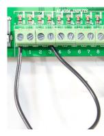
The VoiceOFF can store and play up to 10 audio files via its hard wired alarm inputs or 9999 audio files if you use RS232 commands from another device like the Alien DVR. To playback an audio file, the VoiceOFF is triggered by connecting one of its alarm inputs to a ground. It really is that easy to use the VoiceOFF!
