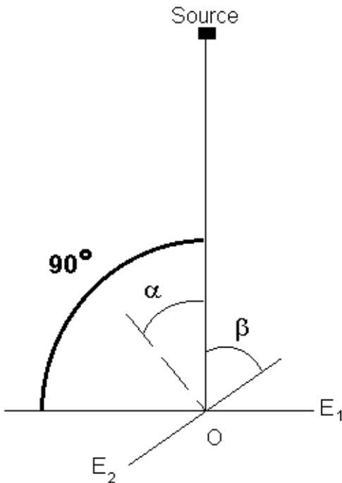
Effective illumination is proportional to the cosine of the angle of incidence of the light on the surface (angle between the direction of the light and the perpendicular to the surface)
