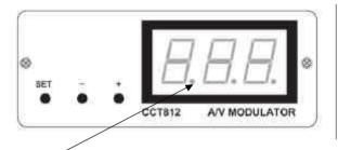
• LED Channel Indicator. When on, this indicates that the actual channel number is 100+ the number on the display.
