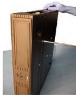
5. Fixing the HDD in the DVR.
