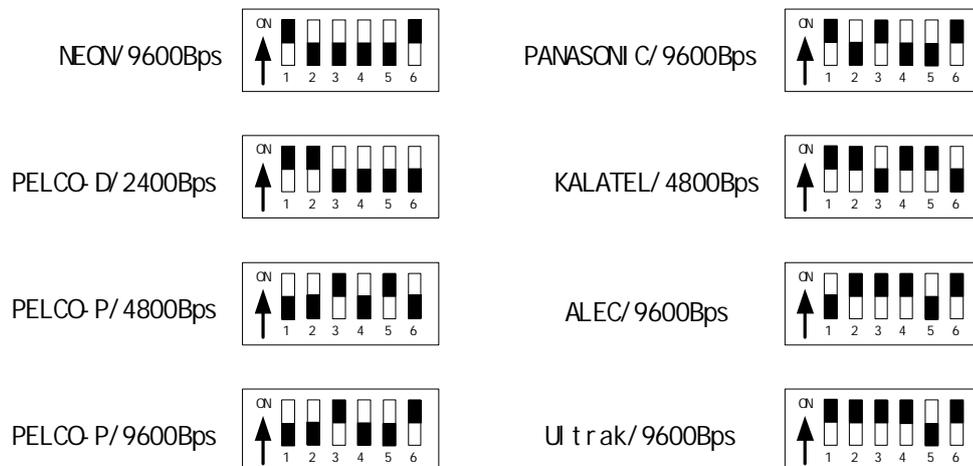
**Setup of the Baud Rate of Communication.**
