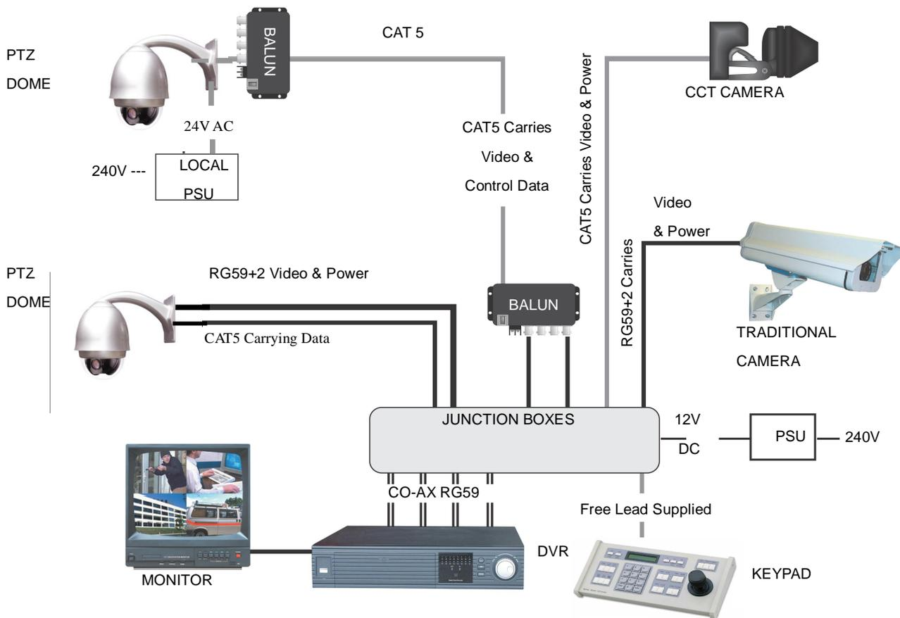
Many installation companies can get the power and video signal correct, but struggle with the control of the dome using the keypad or DVR using the RS485 data.
