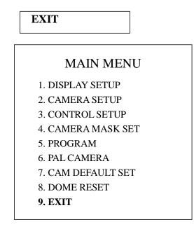
Use the Joystick to select the option and press the CLOSE button to exit menu.
