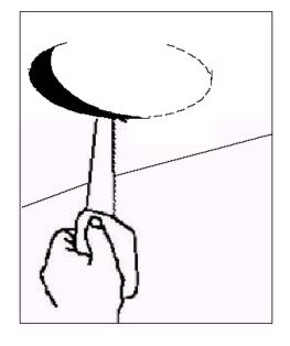
c) Cut out the ceiling material using an appropriate cutting tool (Figure 21)
