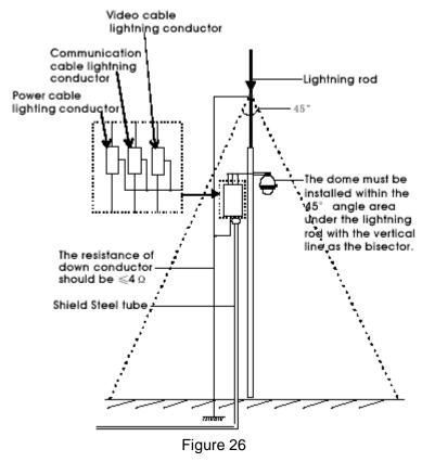
**NOTE:** This technology <u>HELPS</u> prevent the dome and camera from being damaged by lightning strikes but under no circumstances does it guarantee protection. Domes or cameras struck by lightning will not be covered by the warranty.
