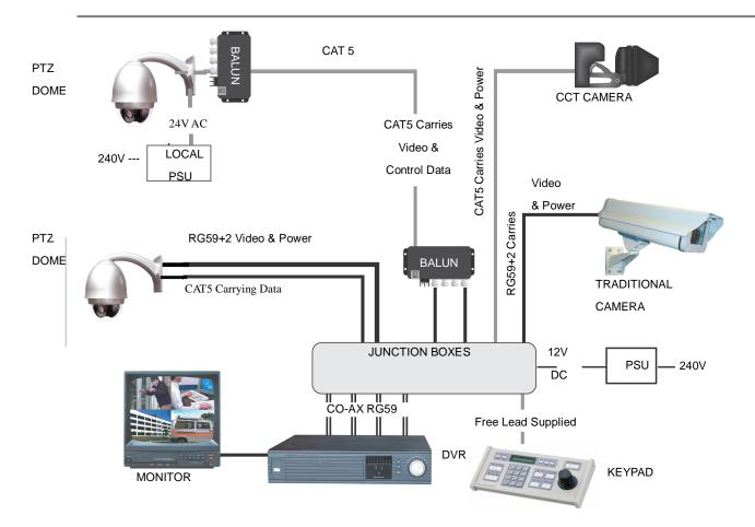
Many installation companies can get the power and video signal correct, but struggle with the control of the dome using the keypad or DVR using the RS485 data.
