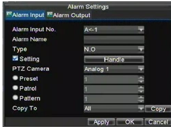
Figure 6. Alarm Management Settings
