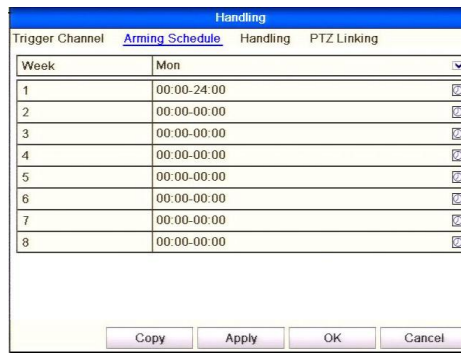
Figure 8.2c Set Arming Schedule for Alarm Input
