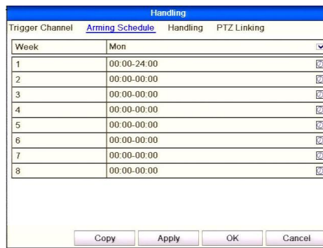
Figure 8.2c Set Arming Schedule for Alarm Input
