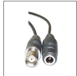
Remember that the Video out from the camera is like any other electrical circuit and requires two wires to complete the circuit. When using a co-ax type cable such as RG59 or similar, the outer braid of the co-ax provides the "0V GROUND" connection and the inner core provides the "Video" connection.
