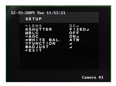
Select the LENS type first. DC for DC Drive Iris Lens, Manual for fixed Iris Lens and Video for Video Drive Iris Lens.
