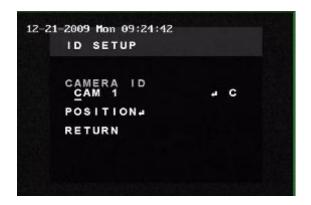
Use the POSITION button by selecting it and pressing set button. Move ID to camera position required and press set button. Click on left arrow button to close and then select RETURN. Note that the camera ID is only displayed when the CAMERA ID is switched to ON.
