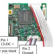
adequate for powering one or two cameras, but when powering more you must look at the bigger power supplies. Using an underrated power supply will cause
