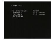
LENS DC/ELC DC 쉰 Direct Drive Lens or ELC 쉰 Electronic Lens
