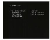
LENS DC / ELC DC 쉰 Direct Drive Lens or ELC싄 Electronic Lens
