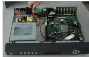
4. Install the HDD. Please note the HDD is placed upside down. Please make sure bracket is in correct position.
