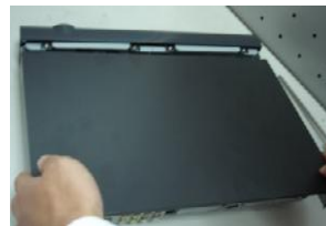
2. Remove the upper cover of the DVR
