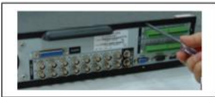
1. Loosen the screws of the upper cover.
