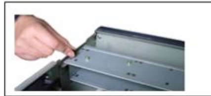
2. Remove the HDD bracket from internal unit.
