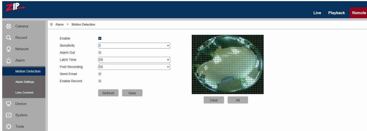
**Enable:**  Click in box to enable motion detection.
