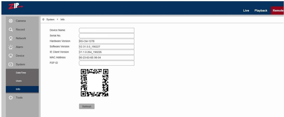
This menu describes the system information held on the camera including the device name, serial number, Hardware Version, Software Version, I.E Client version, MAC address and P2PID. You can use the P2P ID code for mobile phone parameter setup.
