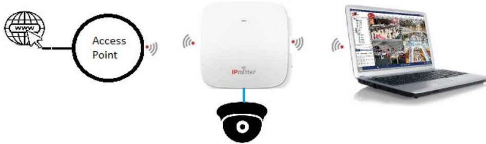
Repeater extending the WiFi coverage and wirelessly adding a camera.
