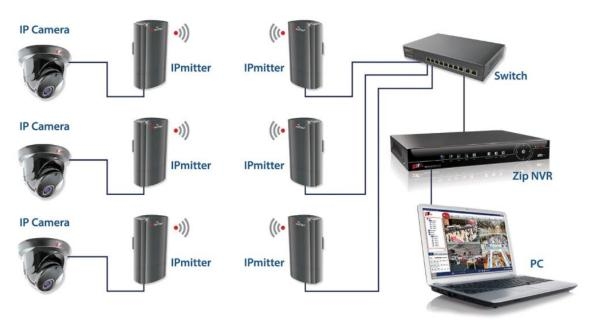
When pairing, the units needs to be set to "Client" and "Host" but with different channel numbers.
