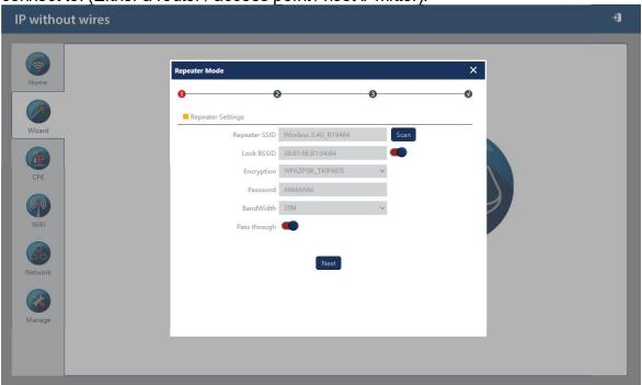
**Repeater SSID** is the WiFi network SSID this IPmitter is to connect to. To find the network you want to connect to press Scan and then select the WiFi network name.
