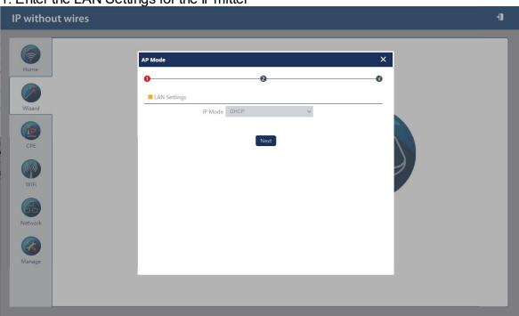
**IP Mode** can be set to either GHCP, static or DHCP. GHCP is set as standard, and will receive an address (similar to DHCP, but will also assign another IPmitter connected to an available address), static IP address is a unique fixed address which you can assign to the IPmitter. DHCP will obtain the address from the DCHP server or the router and assign IPmitter with an address from the network.
