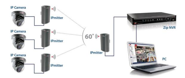
When pairing, one unit needs to be set to "Host" and the many sender units need to be set to "Client".
