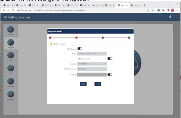
**WiFi Status** controls the WiFi on the repeater. When used purely as an IP camera bridge then it is recommended to leave this option off. When enabled the repeater will broadcast its own WiFi network as well as the existing WiFi network.
