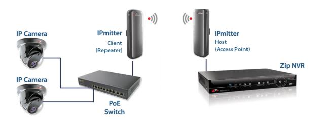
When pairing, one unit needs to be set to "Client" and the other unit needs to be set to "Host".
