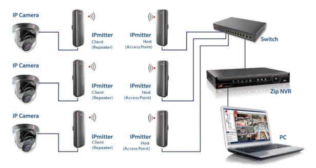
When pairing, the units needs to be set to "Client" and "Host" but with different channel numbers.
