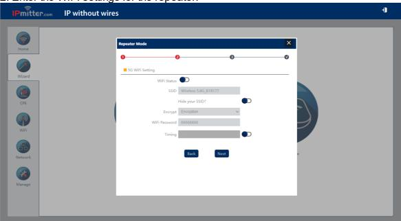
**WiFi Status** controls the WiFi on the repeater. When used purely as an IP camera bridge then it is recommended to leave this option off. When enabled the repeater will broadcast its own WiFi network as well as the existing WiFi network.
