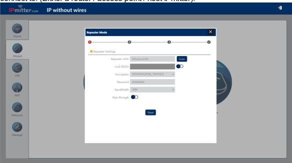
**Repeater SSID** is the WiFi network SSID this IPmitter is to connect to. To find the network you want to connect to press Scan and then select the WiFi network name.
