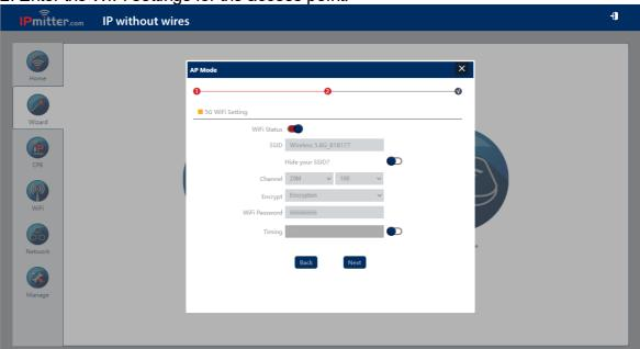
**WiFi Status** controls the WiFi on the access point. When enabled the access point will broadcast its own WiFi network as which extends the LAN connection.
