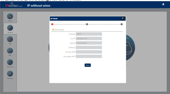
**IP Mode** can be set to either GHCP, static or DHCP. GHCP is set as standard, and will receive an address (similar to DHCP, but will also assign another IPmitter connected to an available address), static IP address is a unique fixed address which you can assign to the IPmitter. DHCP will obtain the address from the DCHP server or the router and assign IPmitter with an address from the network.
