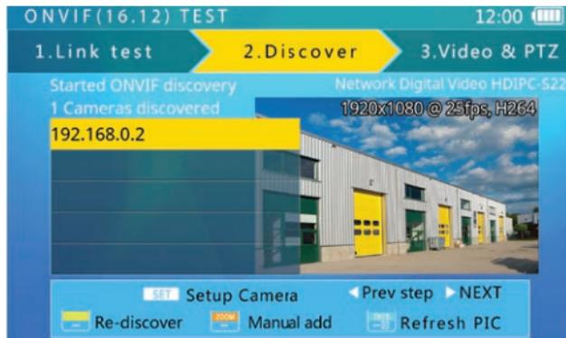
The device list is populated if and when ONVIF devices are discovered. The IP address and/or the device name
