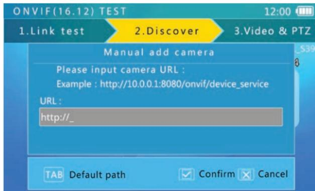
At the '**Manual Add Camera**' screen enter the camera's URL then press the '**IRIS +**' button to confirm.
