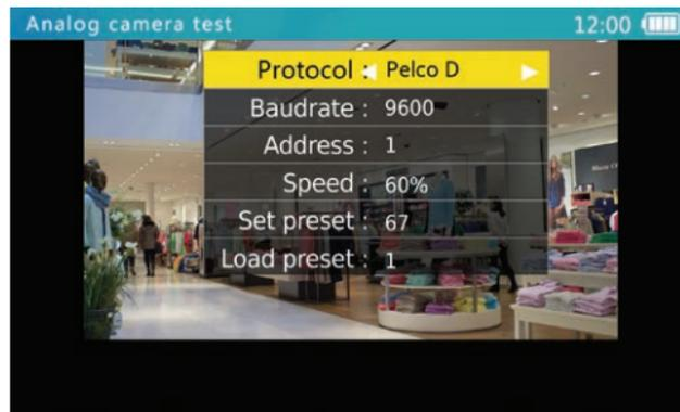
Use the up and down arrows to highlight parameters and the left and right arrows to change values.
