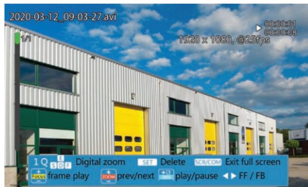
Playback controls are displayed at the bottom of the screen including play/pause, digital zoom and frame by frame playback.
