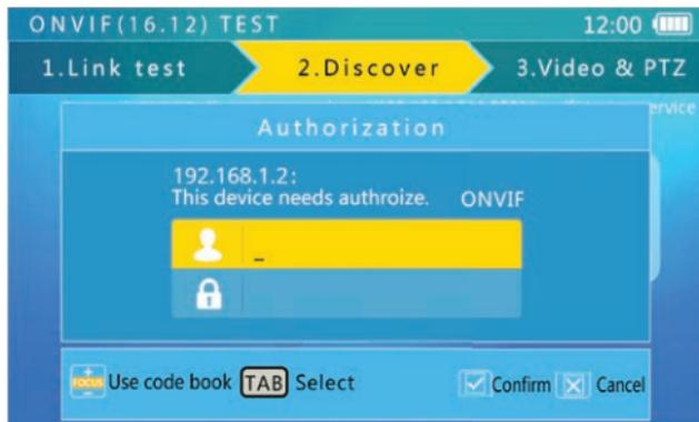
Enter the camera's user name and password then press the '**IRIS +**' button to confirm.
