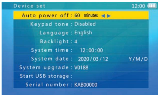
To change settings use the **Up** and **Down** arrow keys to highlight the parameter you wish to configure. Use the **Left** and **Right** arrows to alter the value and then press 'IRIS +' to save changes.
