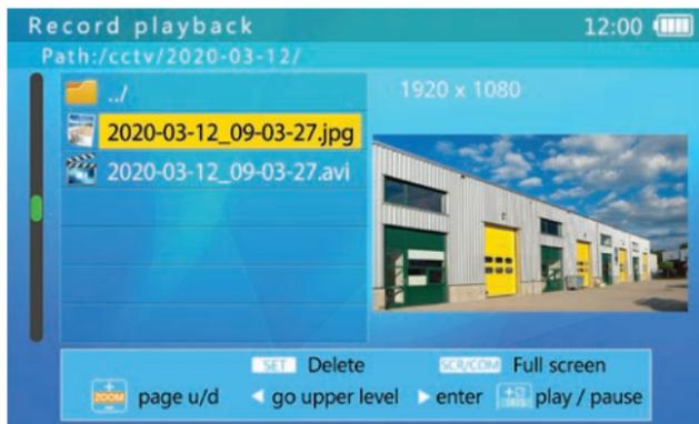
Use the **Up** and **Down** arrow keys to highlight the folder you wish to open. Folders are automatically named with the date on which the files were captured.
