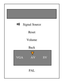
Misc. Signal Source This option allows the signal source to be selected.
