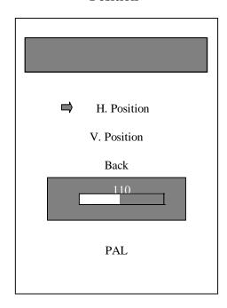
Position This option allows the horizontal and vertical centering of the screen display.
