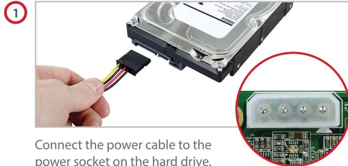
Connect the power cable to the power socket on the hard drive. Connect the other end (White plug) to the power socket on the PCB.
