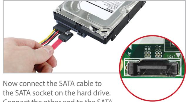
Now connect the SATA cable to the SATA socket on the hard drive. Connect the other end to the SATA socket on the PCB then place the drive in the DVR case.
