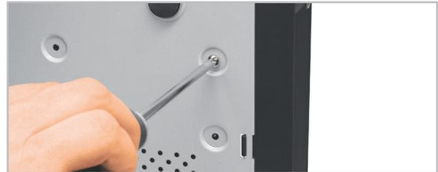
Screw through the four holes in the base of the DVR, and into the four fixing holes in the bottom of the hard drive. (Screws supplied with hard drive.)
