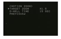
MOTION ZOOM allows the camera to zoom in when motion detected. Note that as most PTZs are in constant movement this camera module option is rarely used.
