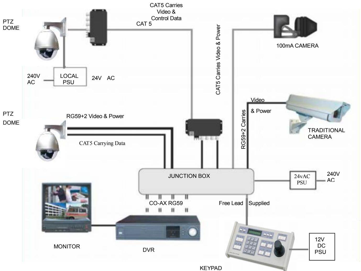
Many installation companies can get the power and video signal correct, but struggle with the control of the dome using the keypad or DVR using the RS485 data.
