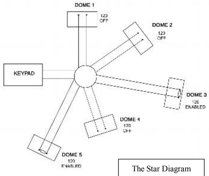
**Overcoming RS485 data loss using an RS485 distributor**
