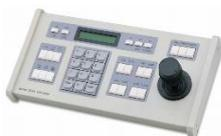
The dome is controlled by an RS485 data signal that is given by either a KEYPAD or a suitable DVR. This data signal tells the dome to pan, tilt, zoom etc. Its important that you read the early section of these instructions to understand the fundamental principle of RS485 cabling techniques so that you get it right.
