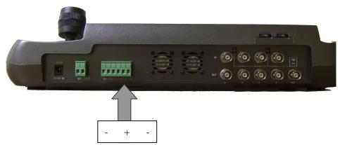
Connect the RS485 data cable to the connections on the rear of the keyboard (see diagram above). Note that the orange connection is the RS485 + A Line connection and the yellow is the RS485 - B Line connection. Note that there are two sets of RS485 connections.
