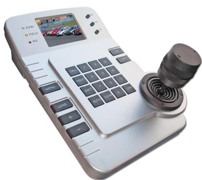
The dome is controlled by an RS485 data signal that is produced by the PTZ715 keypad or a compatible DVR. This data signal tells the dome to pan, tilt, zoom etc.
