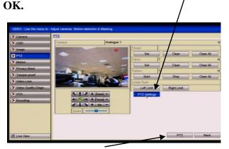
Now click on the **PTZ** button at the bottom of the screen and a full screen picture will be displayed with the PTZ control menu. Click on the **IRIS**+ button to display menu
