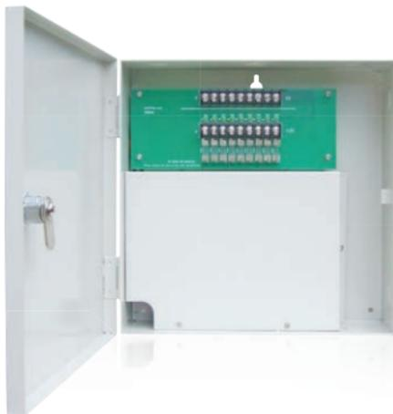
Regulated 12V DC 5 Amp PSU with multiple outputs for use with up to 9 suitable CCTV cameras. Each output produces up to 1 Amp (max 5A overall outputs) to suit most cameras and housings.
