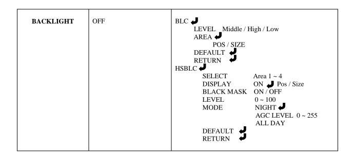
Backlight Compensation when set, can balance light levels during day and night so that light hitting objects viewed, is evenly spread across the picture. There are two options BLC and HSBLC that can be selected.
