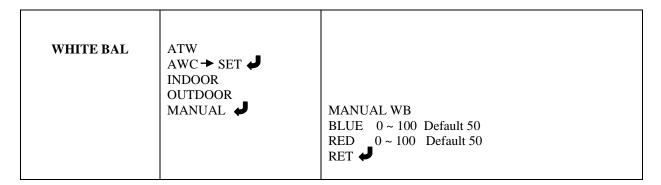
ThE White Balance feature automatically adjusts the colour settings in the camera to match the type of light available, so that white and other colours appear as natural as possible.
