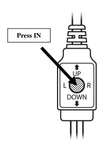
Press the centre button <u>IN</u> (see arrow) to enter the menu and use Left, Right, Up and Down to move through and amend menu settings.
