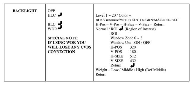
Backlight Compensation when set, can balance light levels during day and night so that light hitting objects viewed, is evenly spread across the picture. There are three options HLC, BLC and WDR that can be selected.
