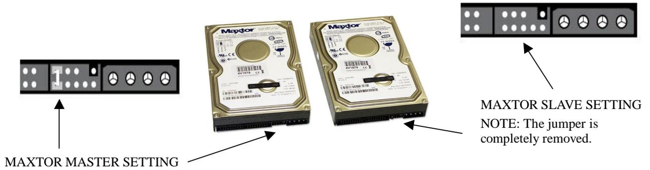
8. Now connect the IDE Ribbon cable and the hard drive power supply plug. These cables have a keyed side so that they can only fit one way round. Note that the ribbon cable has a red edge that faces the red cable of the power supply plug. The left ribbon cable and power plug are for the Master and the right ribbon cable and power plug are used for the Slave.
