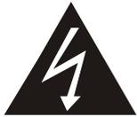
The lightning flash with arrowhead symbol, within an equilateral triangle, is intended to alert the user to the presence of insulated dangerous voltage within the product's enclosure that may be sufficient magnitude to constitute risk of electrical shock to persons.
