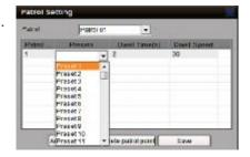
**4th step:** Set the time and speed for the preset. **Note:** Dwell time is between 1 and 128 seconds. Dwell speed is between 1 and 40.
