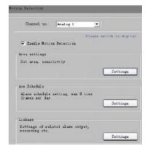
**3rd step:** Set the motion detection area and sensitivity. Sensitivity 1 is lowest and 6 is highest sensitivity level.
