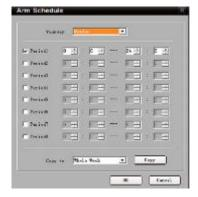
**5th step:** Set the alarm linkage for signal level and select alarm output channel.
