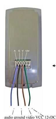
ensuring the wires are connected as shown. Press grey square above wire entry to enter cable.
