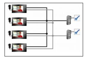
The white 4 core extension cable is approximately 14 metres long. If you need a longer run please note that to avoid voltage drop, you will need to use a heavier cable size as follows:
