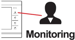
When monitoring a door camera open two way audio by pressing the Talk button.
