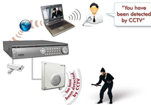
**2** The audio output from the DVR is connected to the yellow audio input phone connector in the VoiceOFF.
