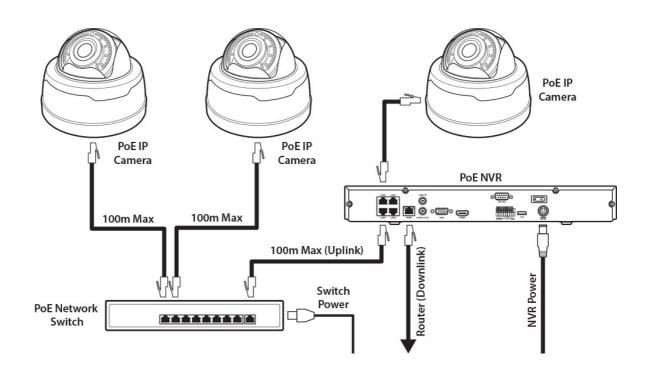
We would usually recommend connecting the switch to the last PoE port to make things easier. This leaves the first PoE ports free for PoE cameras to be connected directly to the NVR.
