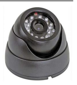
The CAM050 is an attractive internal/external low cost dome style camera with a cleverly engineered three dimentional bracket that allows mounting on walls, ceilings or outdoor structures not possible with two dimentional domes. This day/night dome camera has infra-red leds and switches to black and white mode for better night vision. The dome is anti-vandal resistant and can be used externally without the need for additional enclosures or brackets to protect it.
