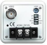
If you are using the System Q Easy Connection Kit (CCT806/7) to power and connect your camera (12V models only) please proceed as per the instructions supplied with The Easy Connection Kit. You will need to cut off the DC Plug ONLY and use the bare wires to connect to the terminal strip. The 12V positive is the RED wire the 0V is the BLACK wire.
