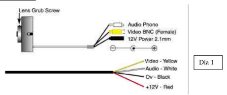
To do this, the camera requires a 12V 100mA+ high quality regulated power supply, a recommended unit is any of the 'ANTIHUM' series of power supplies that are specifically made for getting the best out of CCTV installations. The cameras d.c input connector is a 2.1mm size DC Socket and the middle pin is the 12V+ and the outer case is 0V or ground - please ensure your power supply is regulated and has the same connector configurations or you may damage the camera and void the guarantee.
