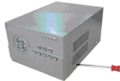
Replace the top cover and fixing screws.
